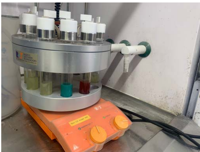
Fig. S1: Parallel reactor employed for the catalytic reactions.
