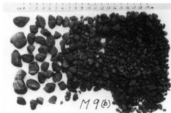
Plate 36: Some samples before and after slake durability cycles
