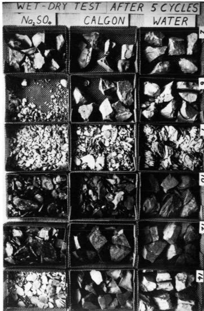
Plate 39: Comparison of the effects of various wetting agents on some of the samples
