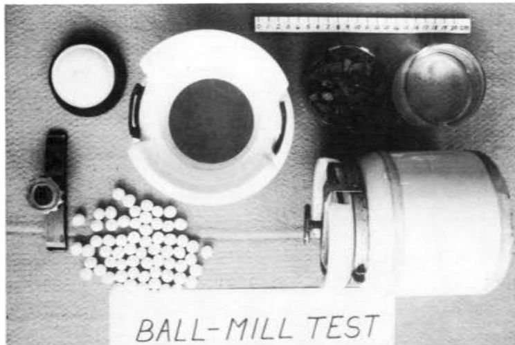
Plate 34: Jars and charge for the wet ball mill test
