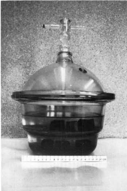
Plate 18: Apparatus used for determining vacuum saturated absorption
