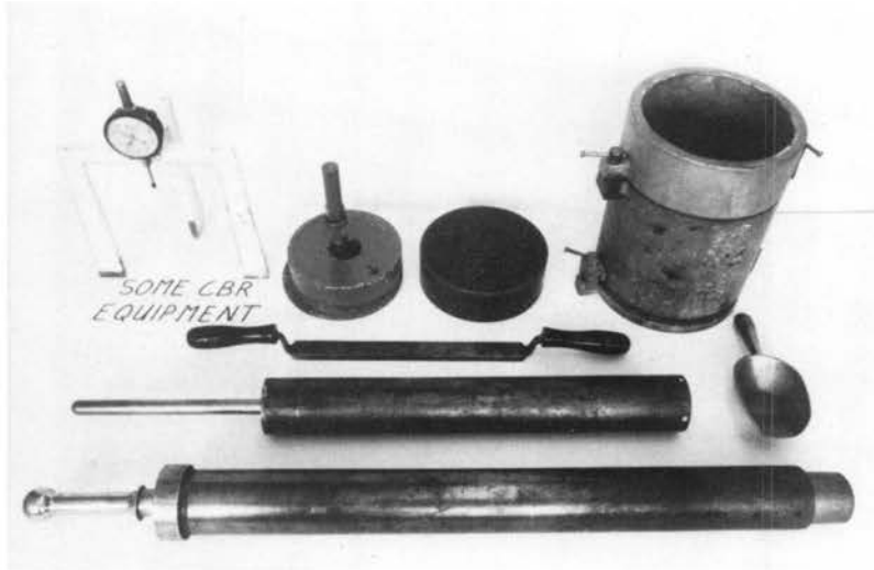
Plate 12: Equipment used for compaction and volume change measurements during the compaction and CBR tests
