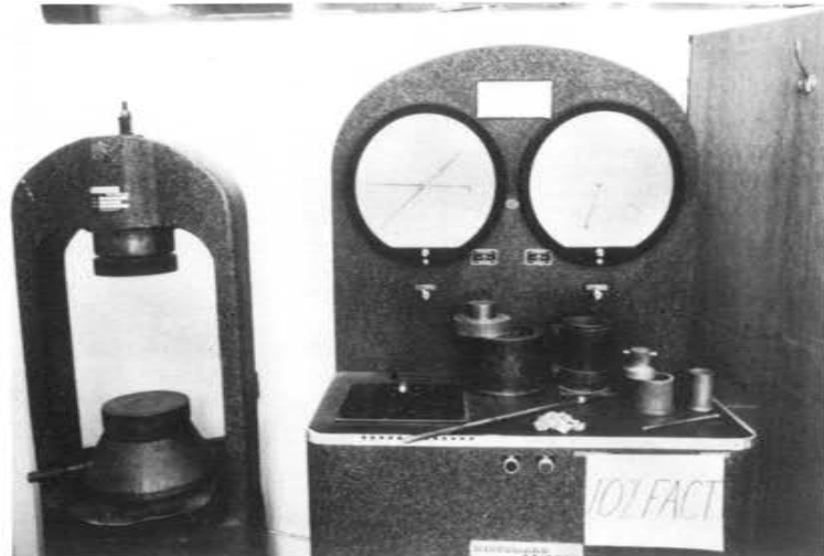
Plate 30: Apparatus for determining the 10% FACT value (large and small cylinders shown)
