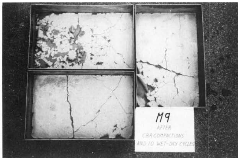
Plate 13: Slaked material of sample M9 after the 1st weathering period (container 320 x 500 mm)
