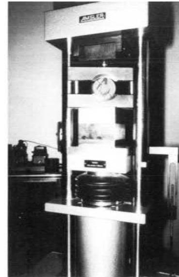
Plate 25: Disk being split during Brazilian tensile strength test
