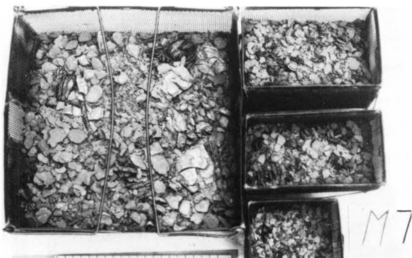
Plate 37: The behaviour of sample M7 during the sodium sulphate soundness test
