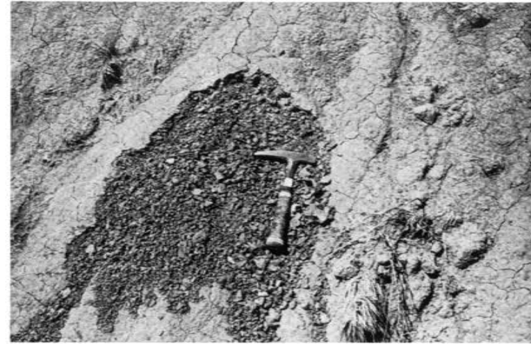
Plate 2: Slaking of mudstone of the Elliot Formation in road cutting between Ladybrand and Clocolan
