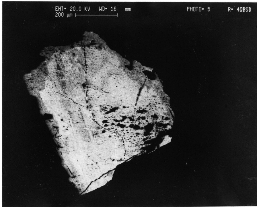
Figure 6: An arsenopyrite crystal, with an As-rich centre, containing numerous inclusions (black), partially surrounded by a S-rich rim - RC 1022 (electron backscatter image)
