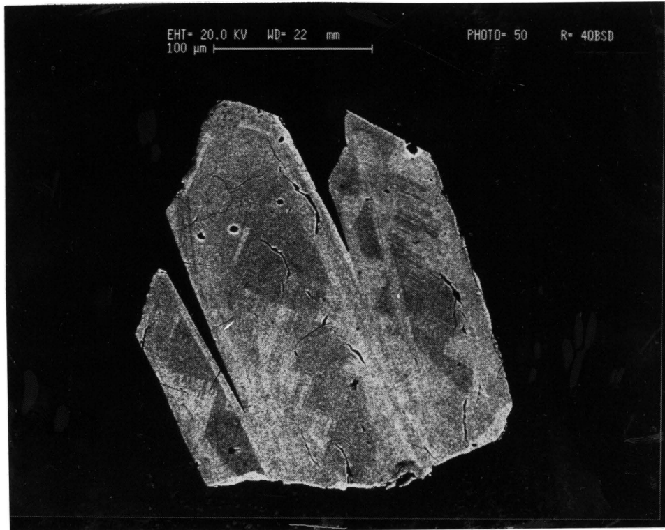
Figure 16: Zoned arsenopyrite crystal, orientated approximately parallel to the c-axis - RC 1026 (electron backscatter image)
