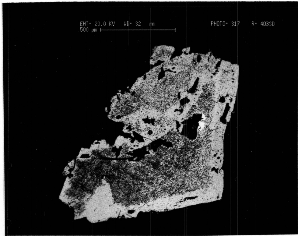
Figure 90: An individual pyrite crystal: (A) before leaching and (B) after bacterial leaching for two days: the influence of composition is shown by extensive pitting within the As-rich areas - RC 1056 (electron backscatter image)
