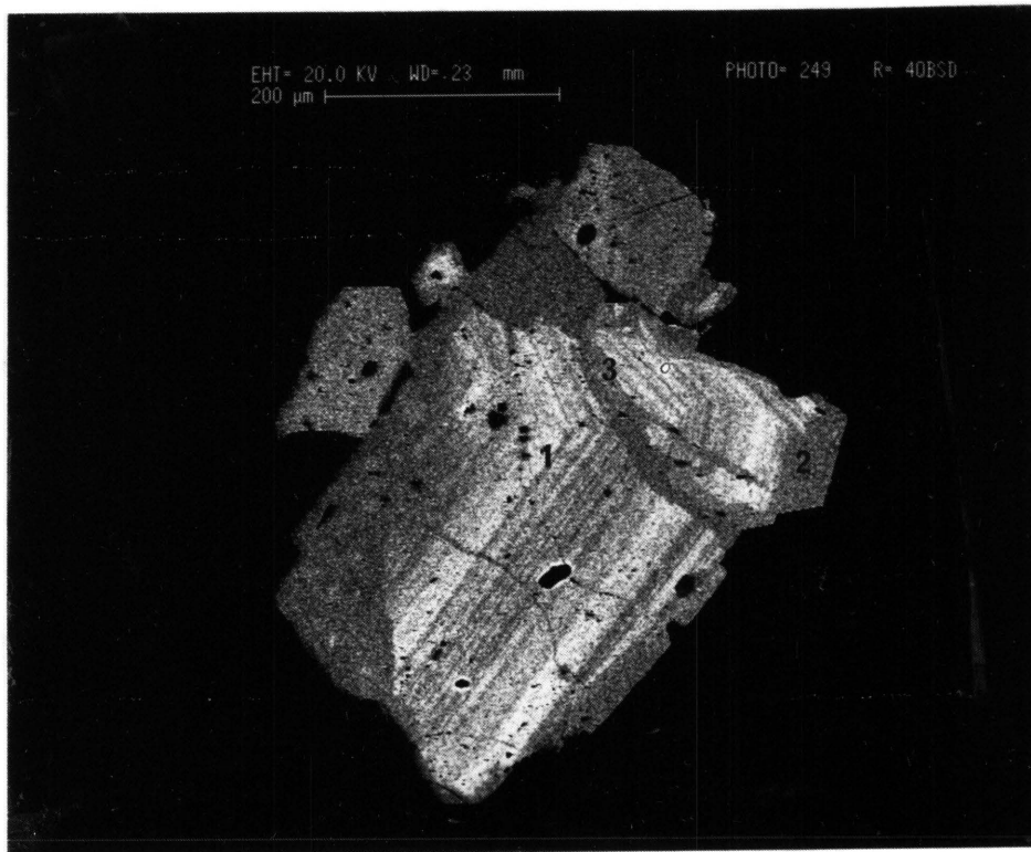
Figure 44: A crystal exhibiting more than one generation of pyrite: the first generation (1) is chemically zoned, the second generation (2) is chemically more or less homogeneous, and the third generation (3) is depleted in As and cuts across the earlier generations.
