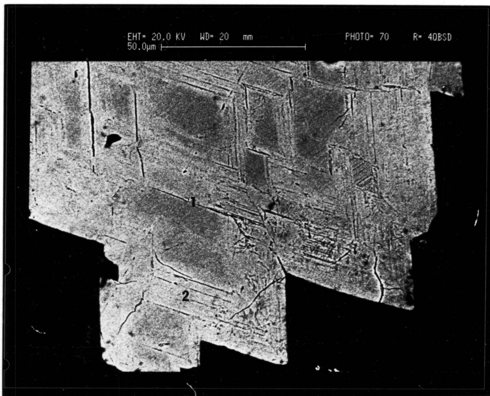
Figure 61: A zoned arsenopyrite crystal after 1 hour of bioleaching - dissolution channels can be seen at the contact between As- and S-rich zones (1) and also within the As-rich zones, parallel to the zone contacts (2) - RC 1018 (electron backscatter image)
