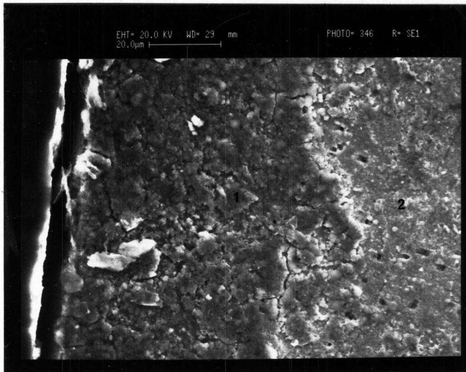
Figure 99: The edge of the crystal shown in Fig. 98: extensive dissolution and disintegration within the crystal edge (1) is visible, while only pit formation is observed in the adjacent intermediate zone (2) - RC 1004 (secondary electron image).
