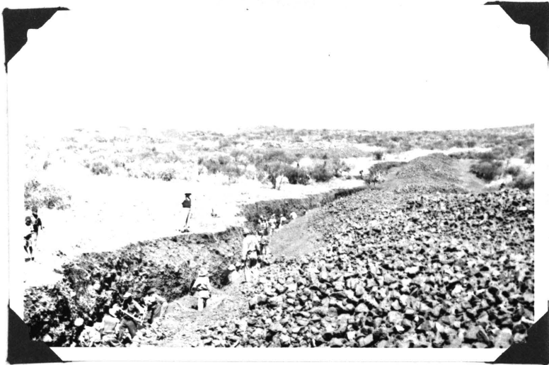
Fig.2. Trench in deposit of ferruginous type manganese ore on Lohathla south. Solid outcrops of ore occur up the slopes to the left of the picture.
