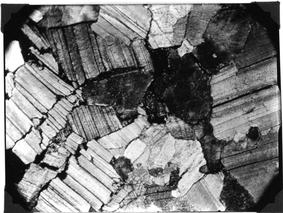
Fig.2. Thin section through a piece of ephesite rock, showing haphazard orientation of individual mica books. Ephesite was formerly termed "pink manganiferous mica" where found on the manganese fields.
