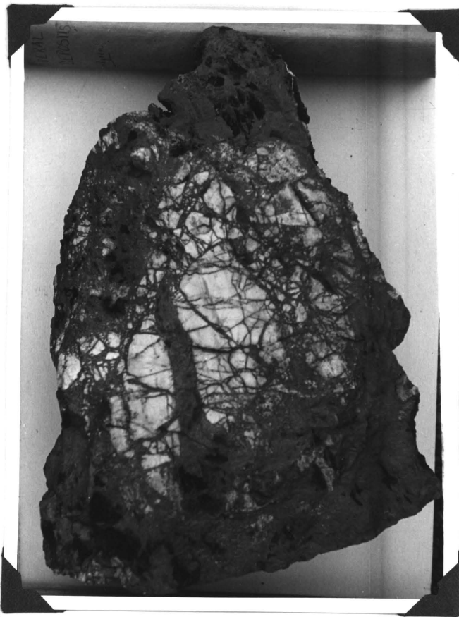
Fig.2. Chert breccia being replaced by manganese, forming "siliceous" type of ore.
