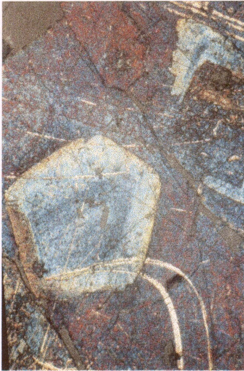
Figure 103. The zoned Sheba pyrite after 9 days in the bacterial leach.
