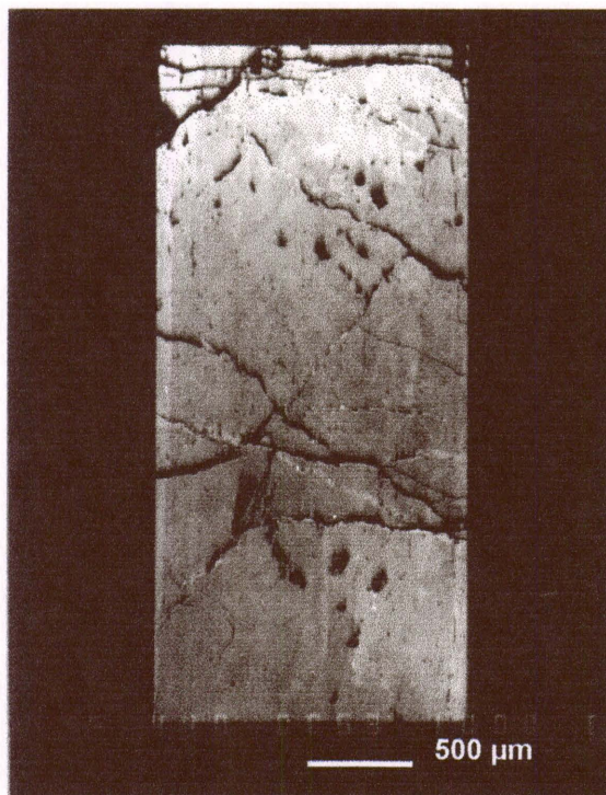
Figure 61. An example of an unusually strongly-zoned Klipwal arsenopyrite. BSE-image.
