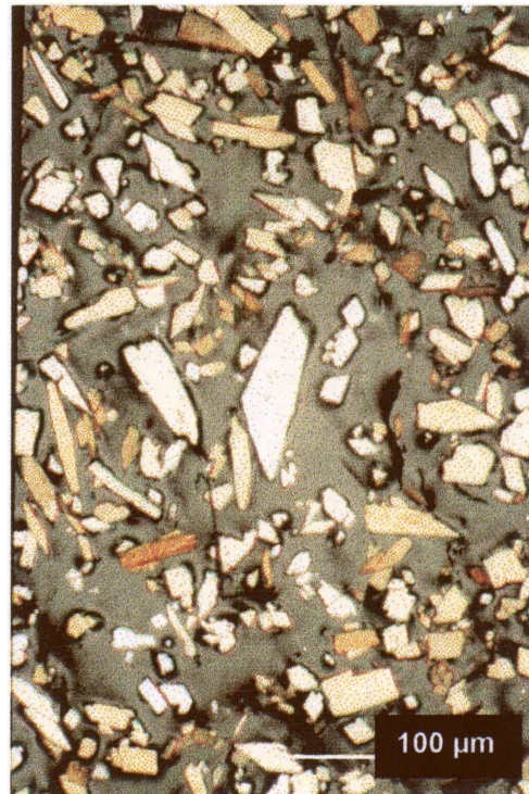
Figure 40. Sheba arsenopyrite crystals after one week in ferric sulphate leach 1.
