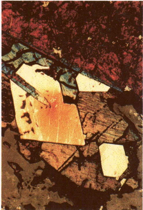
Figure 124. G46 after twelve days in ferric sulphate leach 7.
