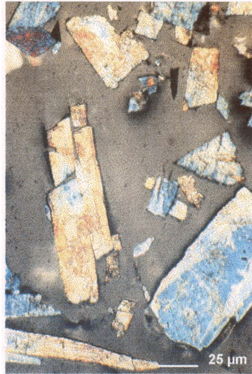
Figure 45. Sheba arsenopyrite crystals after five days in ferric sulphate leach 5.
