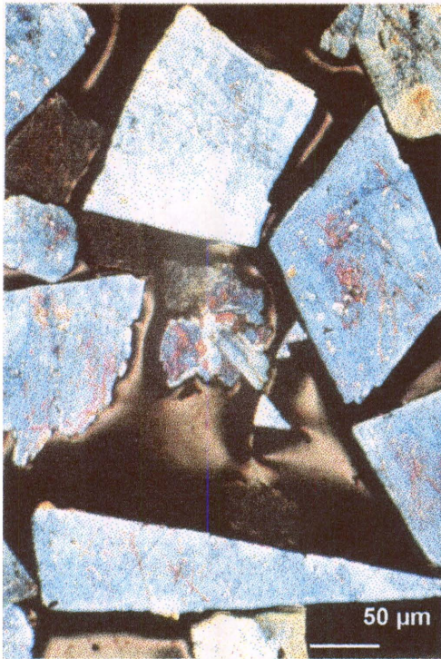
Figure 44. West African arsenopyrite crystals after five days in ferric sulphate leach 5.
