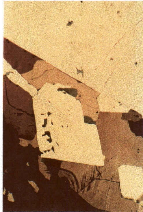
Figure 122. G46 after three hours in ferric sulphate leach 7.
