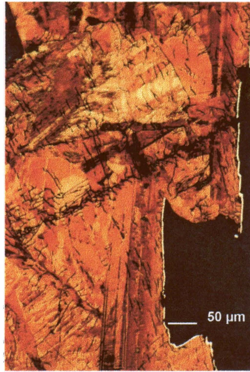
Figure 132. Leach channel development in Zandrivier arsenopyrite after six days in ferric sulphate leach 7. The thin white line is pyrite.
