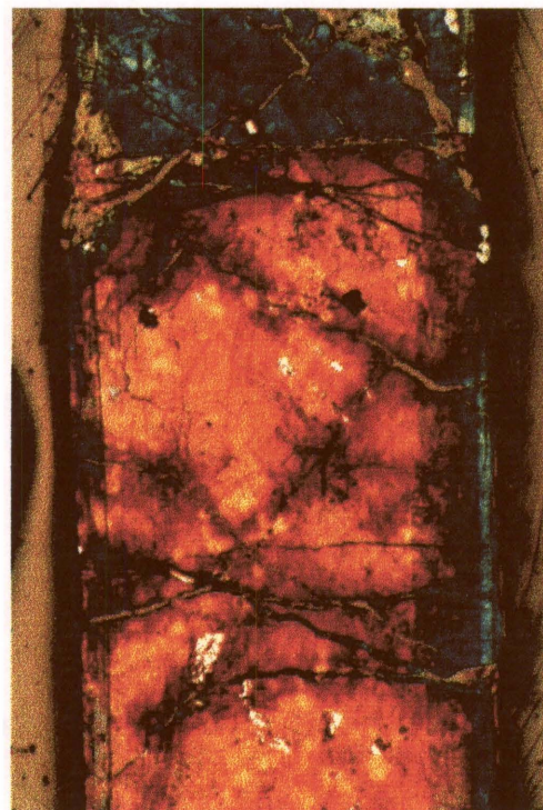
Figure 62. The Klipwal crystal after twelve days in ferric sulphate leach 7.
