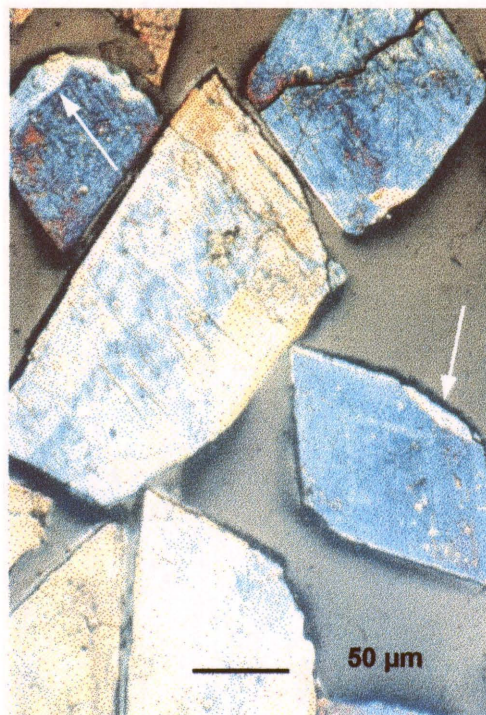
Figure 51. Faster-leaching rims around West African arsenopyrite crystals after one week in ferric sulphate leach 5.
