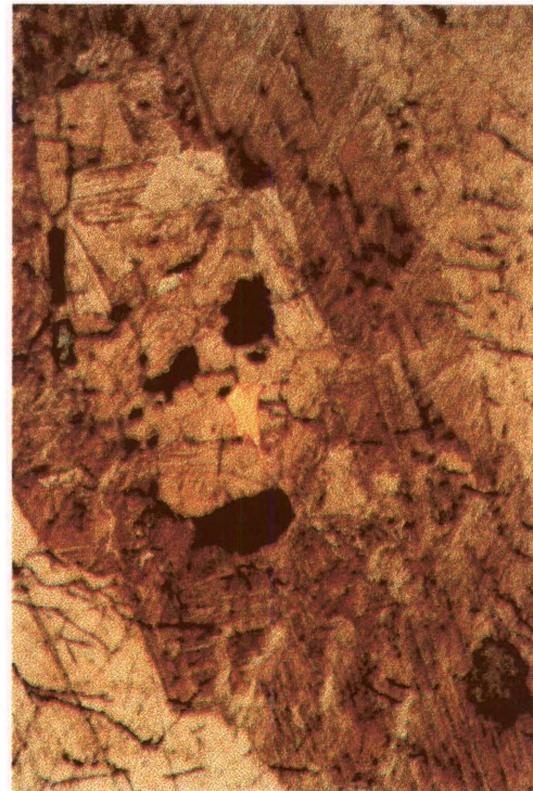
Figure 128. G30 gold after ten days in ferric sulphate leach 7. The gold is unaltered, as is the chalcopyrite, but the arsenopyrite has tarnished and the siderite has dissolved.
