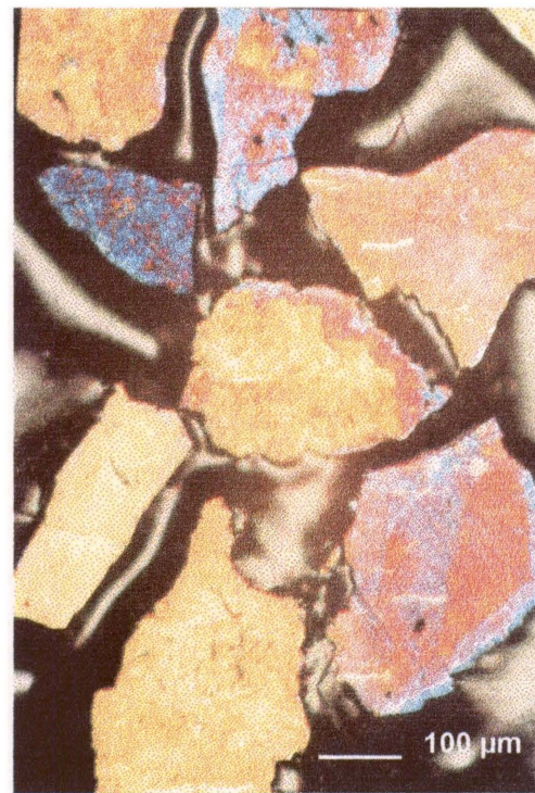
Figure 43. Zandrivier arsenopyrite particles after five days in ferric sulphate leach 5.
