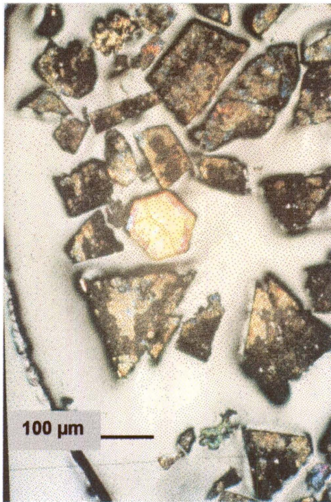
Figure 54. West African arsenopyrite crystals after one week in bacterial leach 1.
