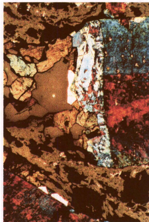
Figure 92. West African arsenopyrite G47A after two weeks in ferric sulphate leach 7.
