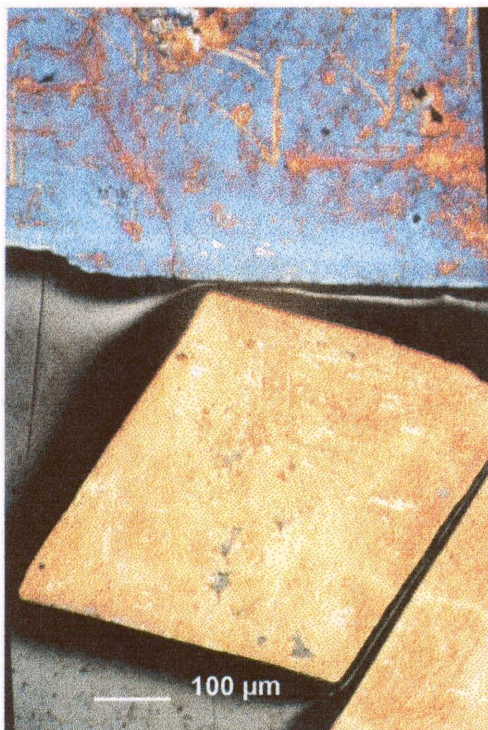
Figure 42. Klipwal arsenopyrite crystals after five days in ferric sulphate leach 5.
