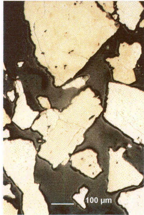
Figure 38. Zandrivier arsenopyrite particles after one week in ferric sulphate leach 1.
