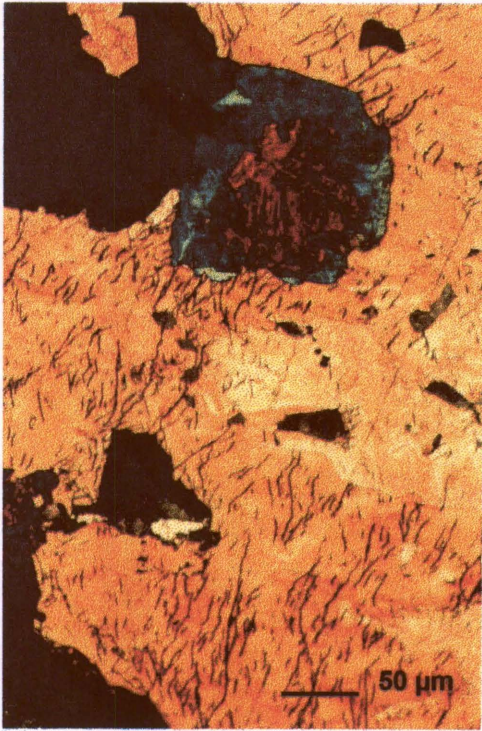
Figure 131. Leach channel development in Zandrivier arsenopyrite after six days in ferric sulphate leach 7. The blue and red areas are also arsenopyrite, but of a different orientation.
