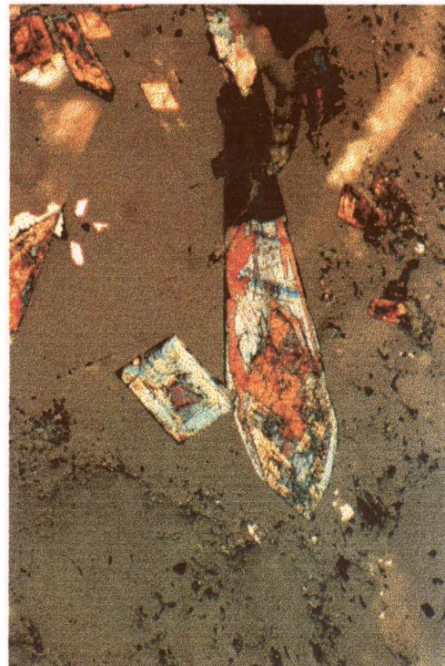
Figure 79. Sheba arsenopyrite crystals A8 and A9 after two weeks in ferric sulphate leach 7.
