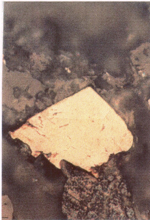
Figure 99. West African arsenopyrite G51 after six days in bacterial leach 3.
