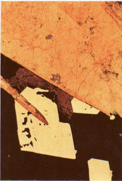
Figure 123. G46 after two days in ferric sulphate leach 7.
