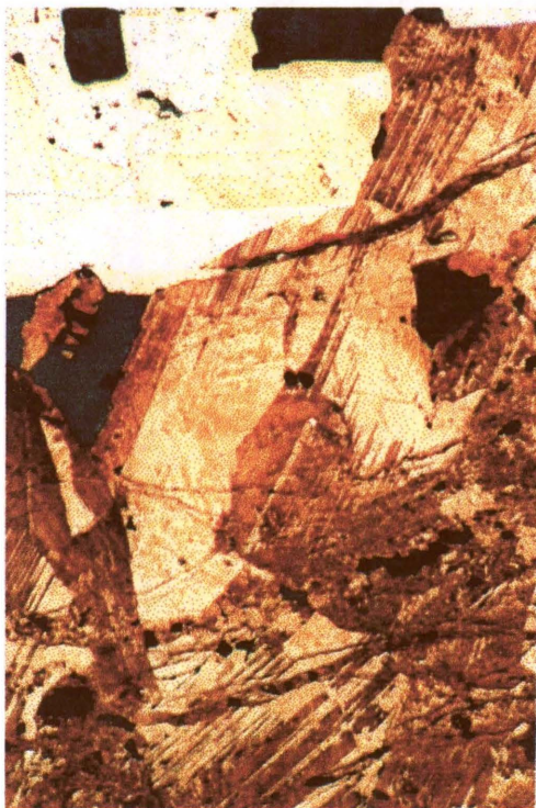
Figure 66. Zandrivier arsenopyrite A28 after two days in ferric sulphate leach 7.
