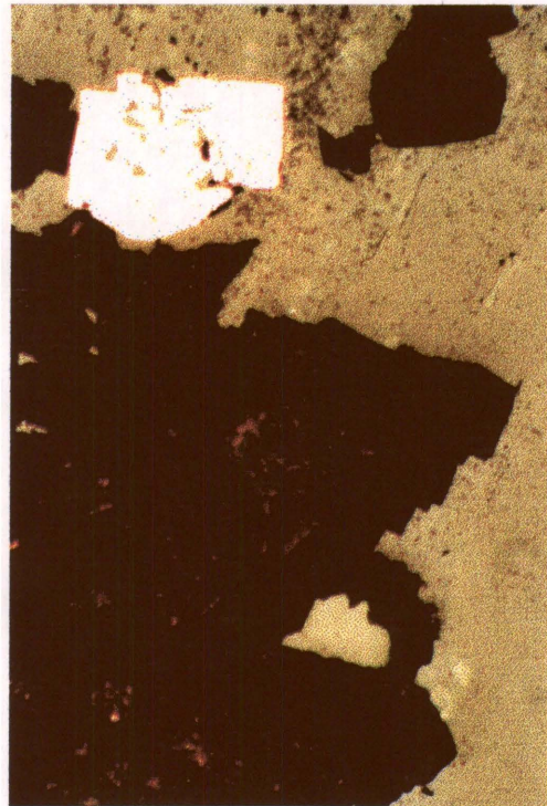
Figure 108. G37 pyrite/arsenopyrite after a week in bacterial leach 3. The arsenopyrite is well-leached, but the pyrite is still untarnished.
