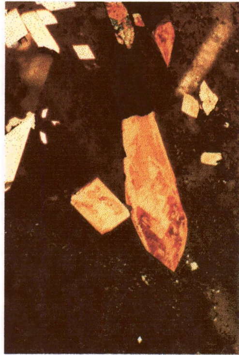
Figure 77. Sheba arsenopyrite crystals A8 and A9 after two days in ferric sulphate leach 7.
