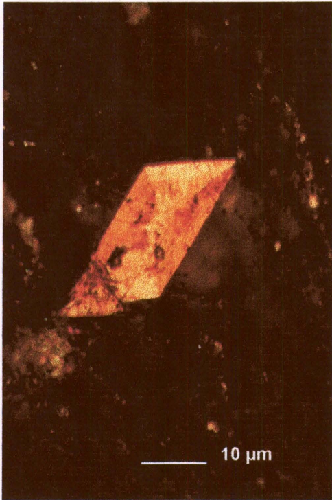
Figure 48. Mimetic twinning apparent in plane light in a Sheba arsenopyrite crystal after six days in ferric sulphate leach 5.
