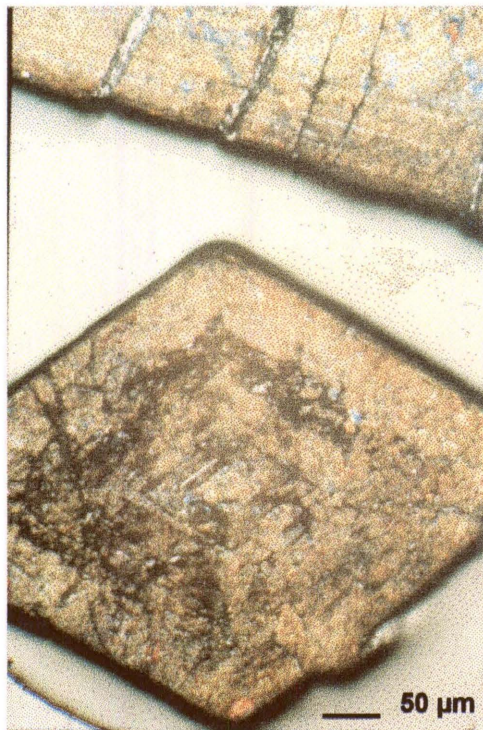
Figure 52. Klipwal arsenopyrite crystals after one week in bacterial leach 1.
