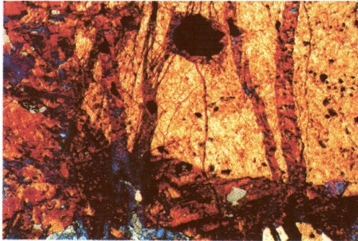
Figure 70. Zandrivier arsenopyrite A30 after eight days in ferric sulphate leach 7.
