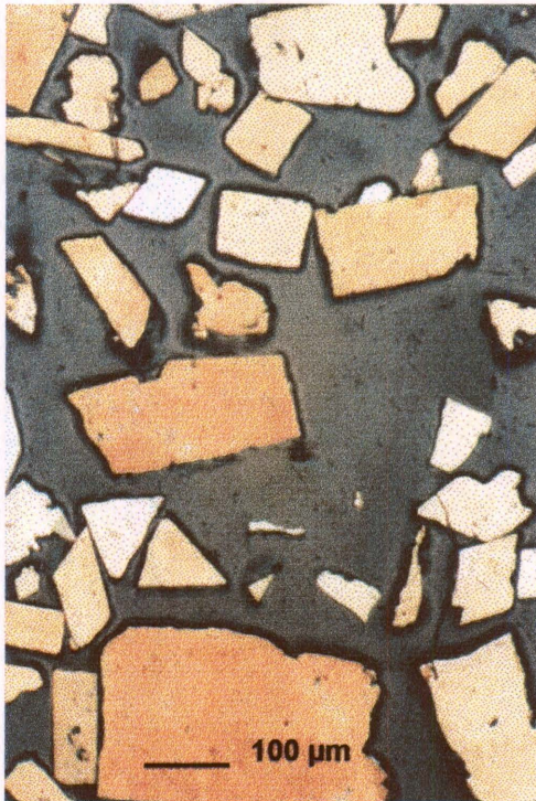
Figure 39. West African arsenopyrite crystals after one week in ferric sulphate leach 1.
