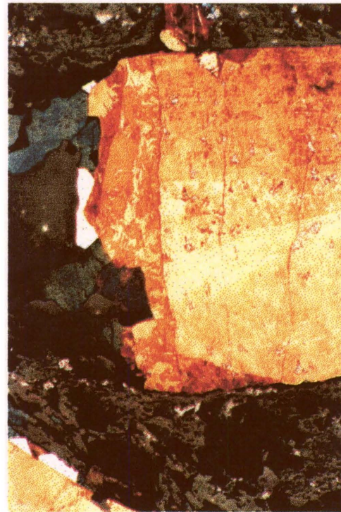
Figure 90. West African arsenopyrite G47A after two days in ferric sulphate leach 7.
