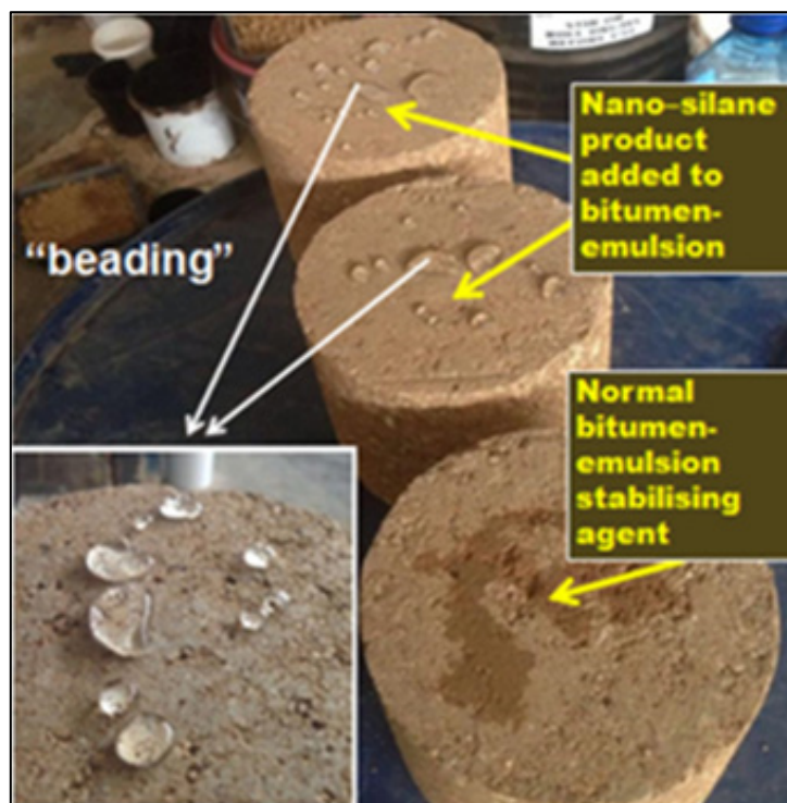
Figure 9: Demonstration of water phobic characteristic achieved with nano-silane treatment (Jordaan & Steyn, 2020)
