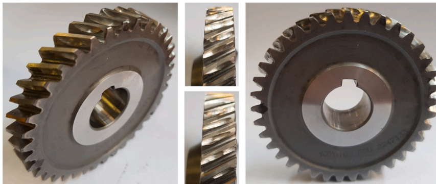
Fig. 15. The gear with distributed damage (case 2) is shown. The gear in Fig. 12 was reused, but the teeth's damage increased.
