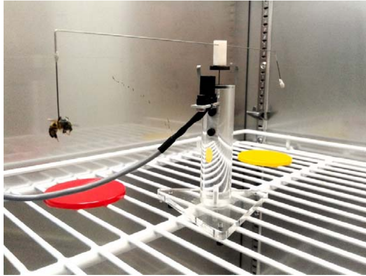
Supplementary Figure 1: Flight mill with honey bee forager attached.
