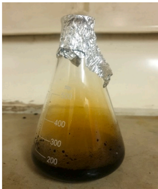
Fig. 14. Pictorial image of tyre crumb pre-treatment showing the yellowish-brown gas emitted during the process.
