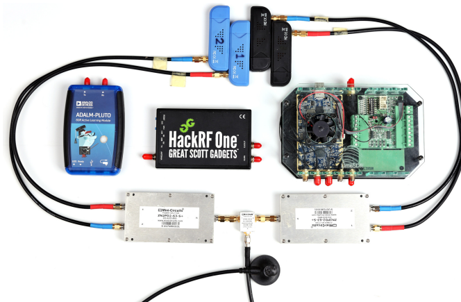
Fig. 2. The hardware used for the experiments showing the SEI receiver antenna at the bottom, the three splitters above it, the three replay-attack SDR devices between the splitters in the middle, and the four RTL-SDR receivers used by the SEI system at the top.
