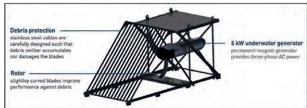
Figure 12. Kinetic turbine for deployment in canal (SHP SMART free stream turbine) (SHP, 2017)
