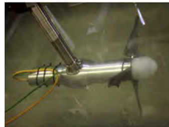
Figure 3-29: Liverpool turbine test setup (Mason-jones, 2010; Morris, 2014)
