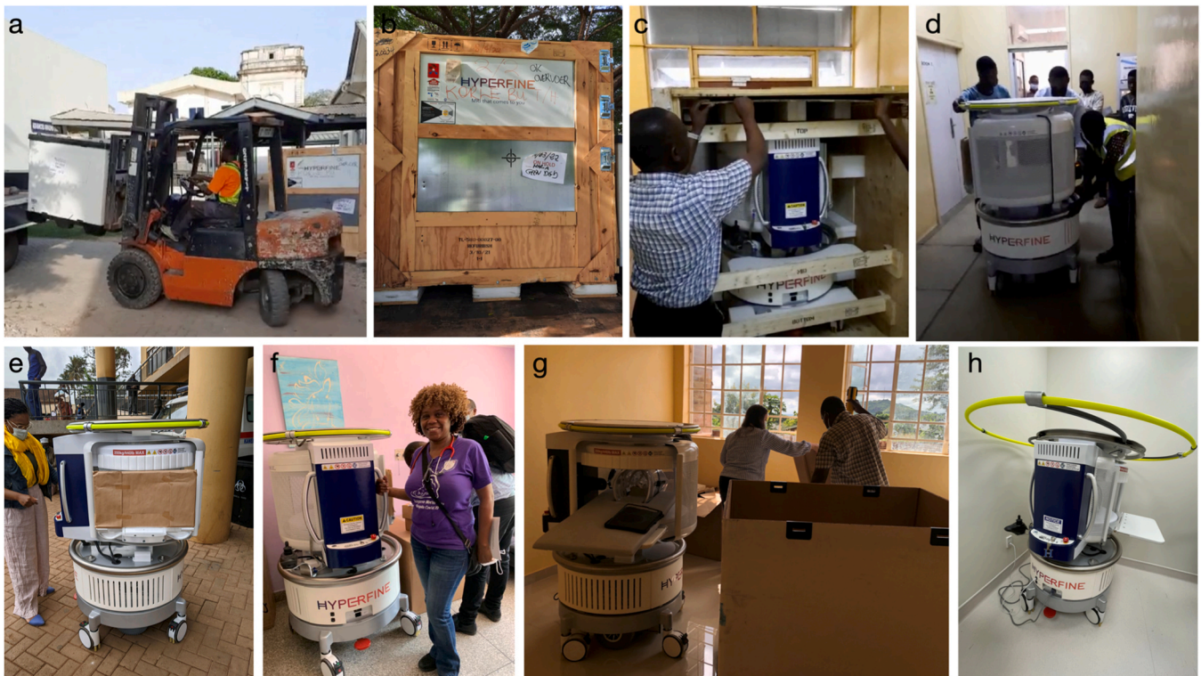
Fig. 5. Pictures of Swoop arriving at a clinical cohort site. Following unloading of the scanner and accessory crate (a and b), the scanner crate is opened and protectors removed (c). The scanner can then be driven out of the grant and into the facility (d, e, and f) to its desired location. Here final set up and unpacking is performed (g) before being ready to image. From arrival to set up can take between 30 and 60 minutes depending on access and distance from delivery point to final scan room.
