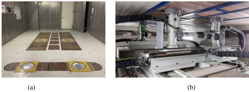
Figure 6. (a) Semi-anechoic chamber in which vehicle is placed on the 4-poster test rig; (b) Room below the floor of the semi-anechoic chamber housing the actuators.
