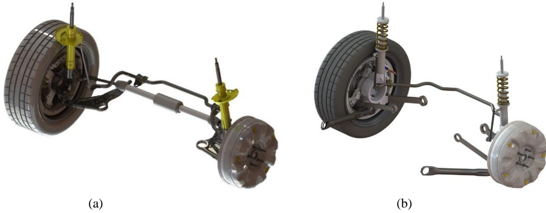
Figure 8. Vehicle corners with in-wheel motors on (a) front suspension and (b) rear suspension
