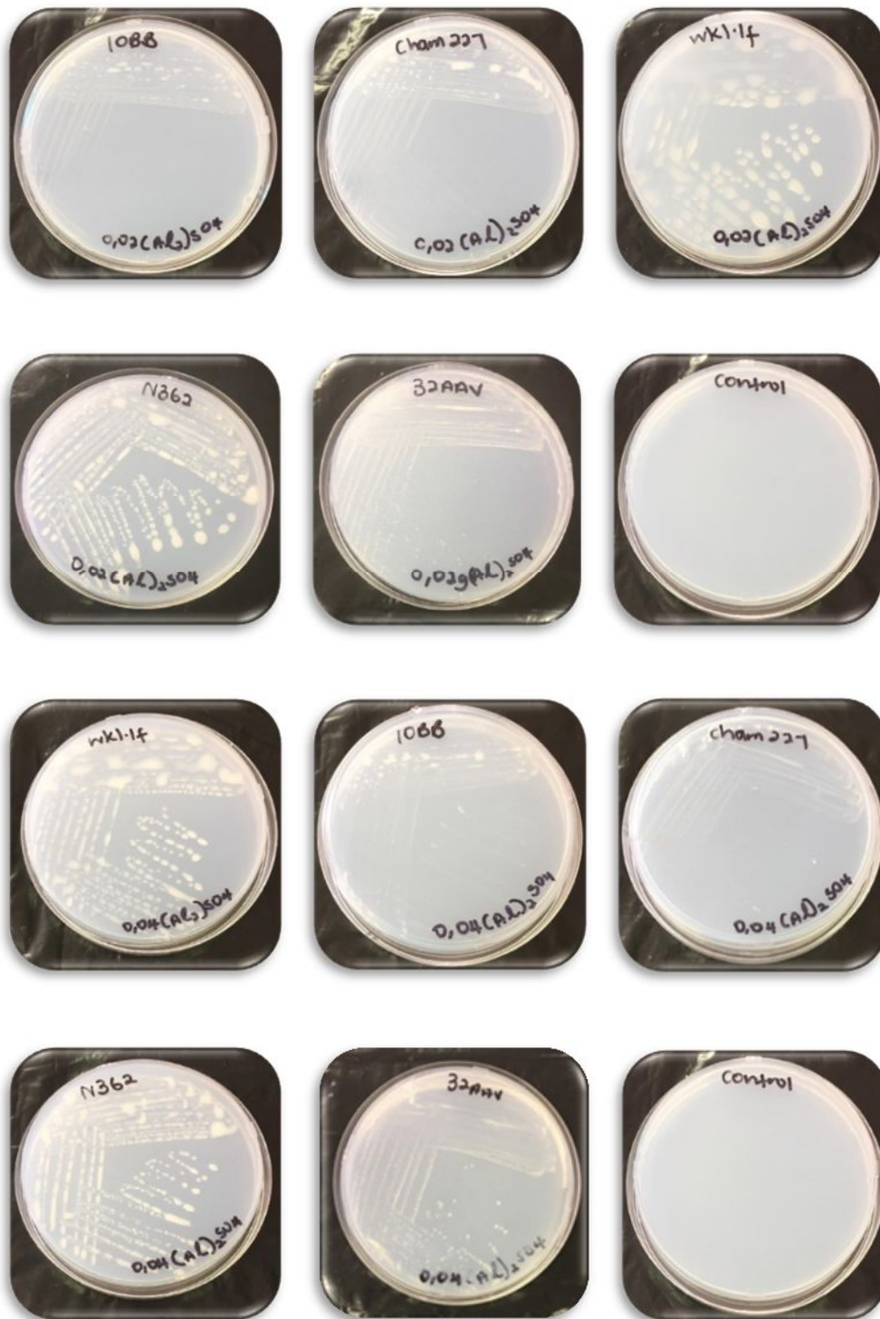
Figure 5. Detection of tolerance to aluminium toxicity of the bacterial isolates when grown under different concentration of aluminium on Keyser's defined medium.
