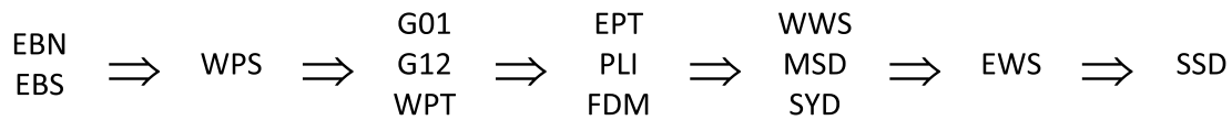
Fig. 10 Increasingly evaporated stable isotope values for sample sites (see Fig. 2). The two exploration boreholes, west of the active mining area, are most similar to meteoric water, followed by mostly groundwater samples and then mine water samples
