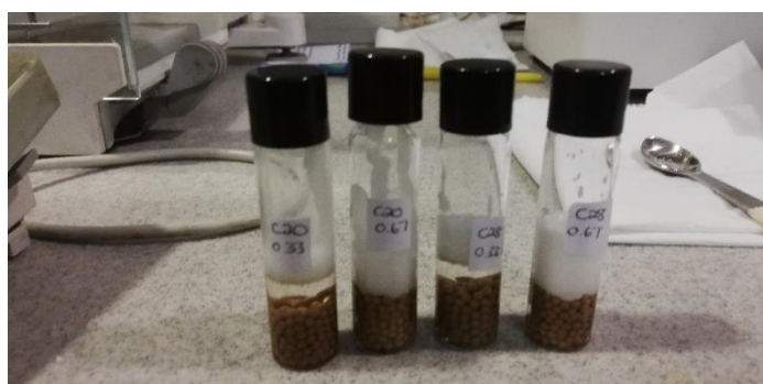
Figure 19: Solid eicosane or octacosane on top of a liquid DEET layer at room temperature.
