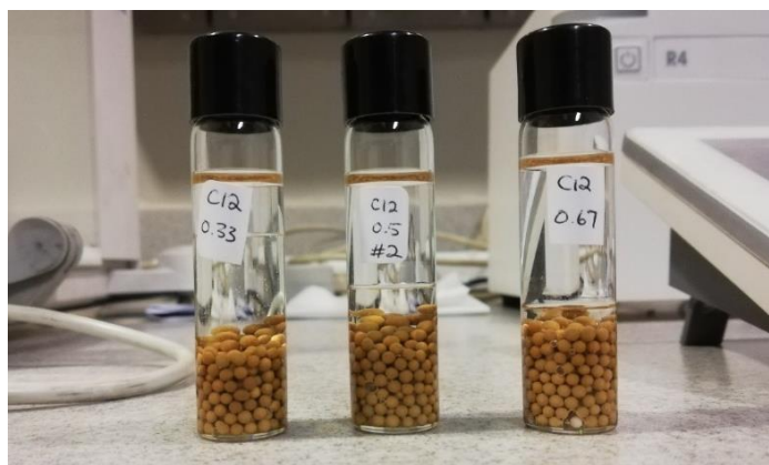
Figure 18: Heterogenous dodecane-DEET mixtures after cooling with two liquid layers.
