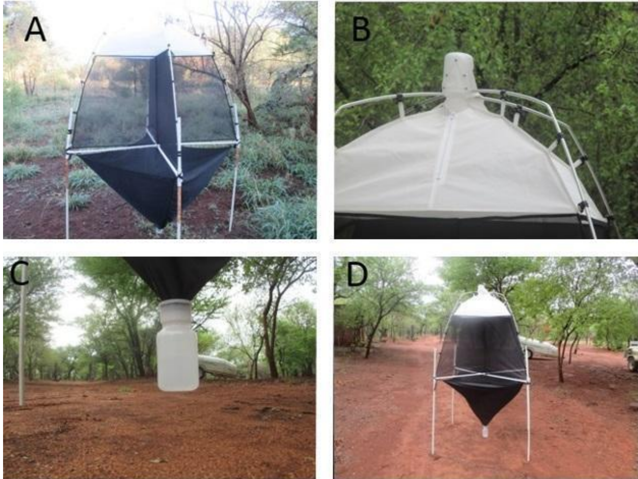
Figure 2.2.3: Malaise intercept trap deployed in the field. (a) A special PVC frame was designed and constructed to allow for deployment in open areas that lack tree anchorage. (b) Top collecting section collected arthropods which flew up in the jar (beneath the zipper). (c) Bottom collecting section collected falling arthropods in the connected jar. (d). Malaise intercept trap with top and bottom jars connected. The top trap has four panels which intercept at the centre.
