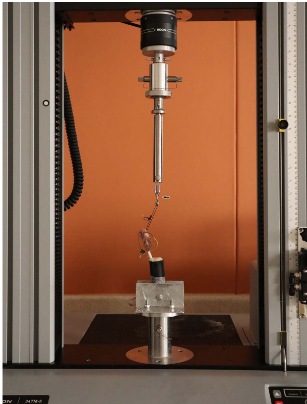
Figure 2 —Positioned specimen for biomechanical testing. The femurs were positioned at a 70° angle relative to the base of the machine. The femoro-fabella ligament suture was placed and connected to a load bar (black arrow) to perform the mechanical test.
