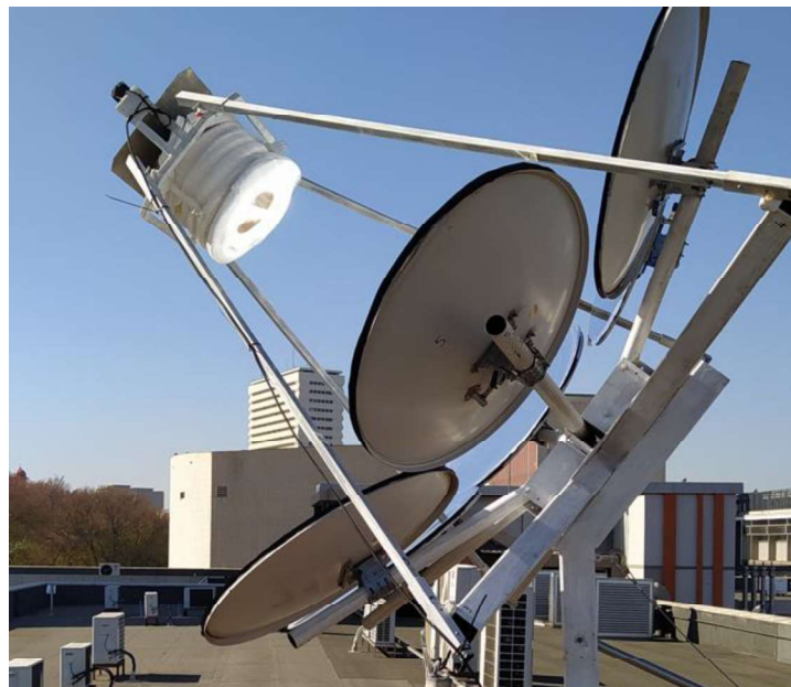
Figure 23. Installed receiver fitted with insulation material and connected to the drive system.
