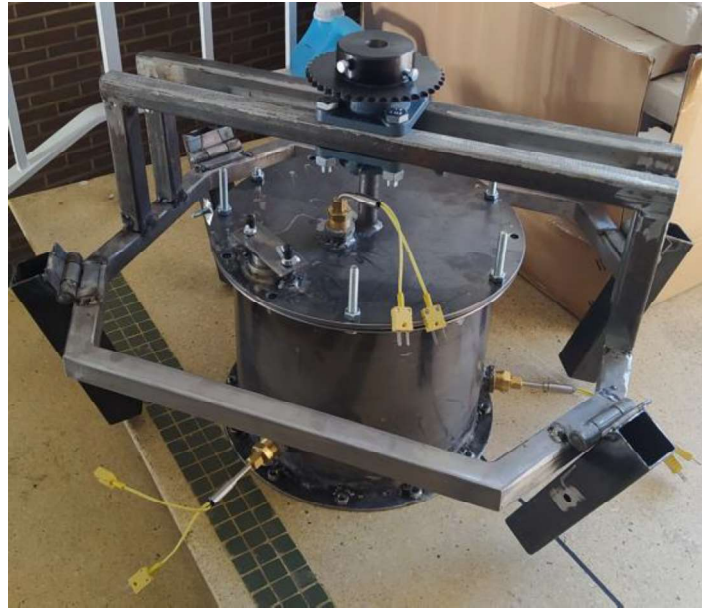
Figure 22. As-built receiver assembly installed in the receiver support frame.
