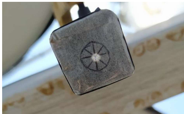
Figure 26. The pin-hole tracker showing a light spot within the 1^\circ target.
