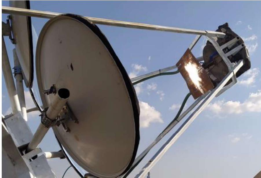
Figure 20. Facet calibration method using the water-cooled plate.
