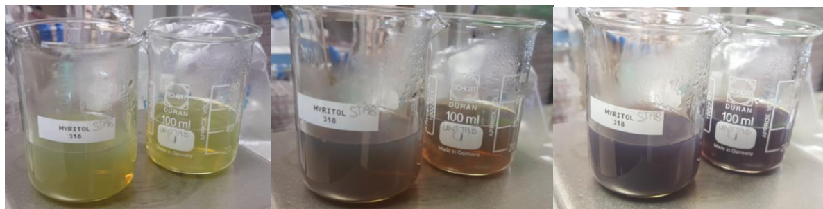
Figure 7.1 Visual inspection of the colour change as the formation of gold nanoparticles with LS and gum arabic progresses. This is the reduction of \text{Au}^{3+} to \text{Au}^0 in the \text{HAuCl}_2 \cdot 3\text{H}_2\text{O} solution turning the solution from yellowish pale green to a dark purple brown colour. The dark purple brown colour is characteristic with the formation of gold nanoparticles within the solution.
