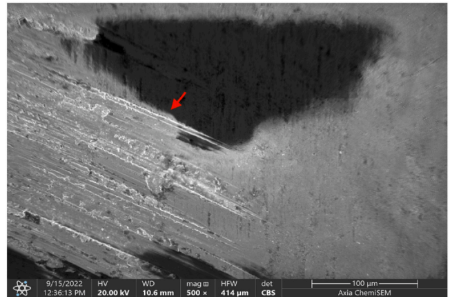
Figure 2. Scanning electron micrograph showing surface scratches (arrow) made on zirconia specimen by super coarse diamond rotary instrument. (Axia ChemiSEM; Thermo Fisher Scientific Inc). Original magnification \times 500 .
