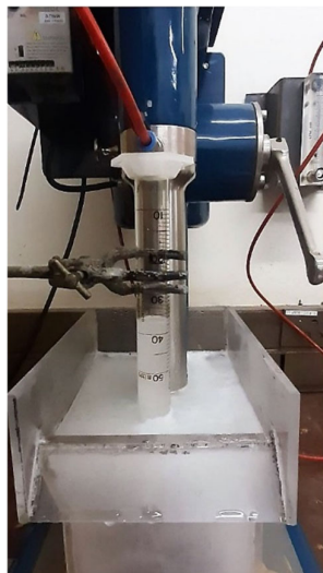
Figure 27: Illustrates the displacement method of measuring J_g .
