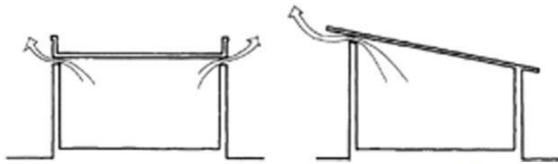
FIGURE 16.98 In the case of pitched roofs, the opening should be in the higher wall.
