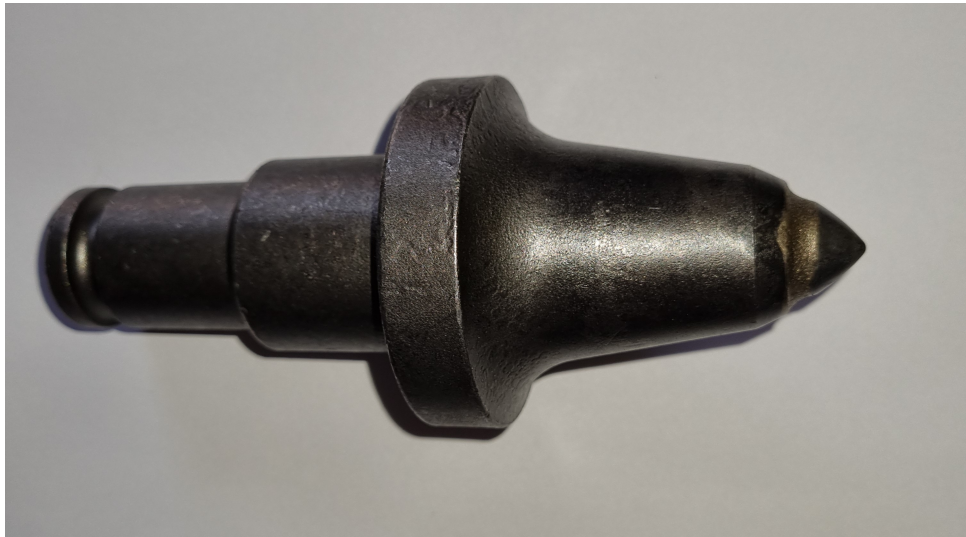
Figure 3.5: Conical pick used in this study.
