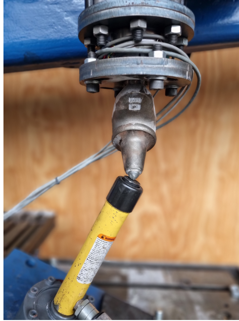
Figure 3.11: Combination of drag force and normal force.
