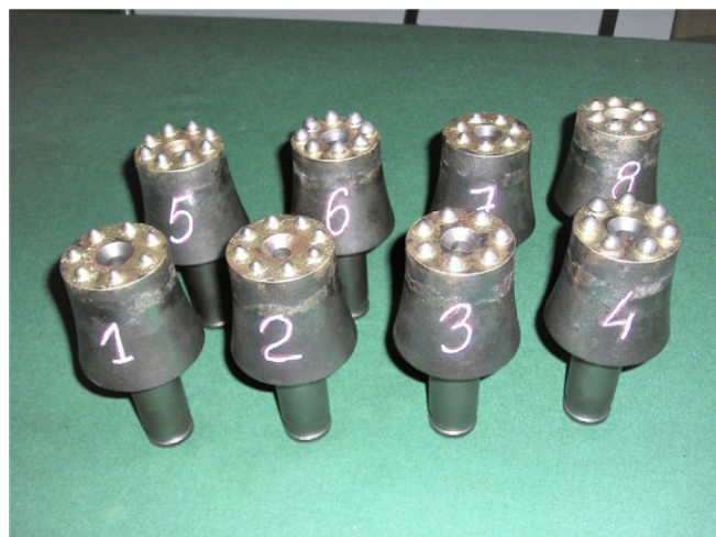
Figure 1.18: Crown picks with different design parameters (Kotwica, 2018)
