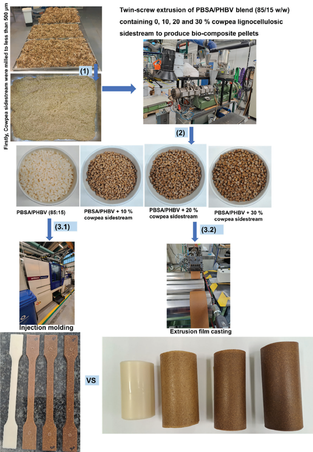
Figure 1. Processing steps to produce injection molded bio-composites and bio-composite films containing 0, 10%, 20%, and 30% cowpea lignocellulosic sidestream. Step 1 shows the milled cowpea sidestream, step 2 shows the compounding of polymers and fibers to produce bio-composite pellets; step 3.1 shows injection molding, and step 3.2 shows extrusion film casting.
