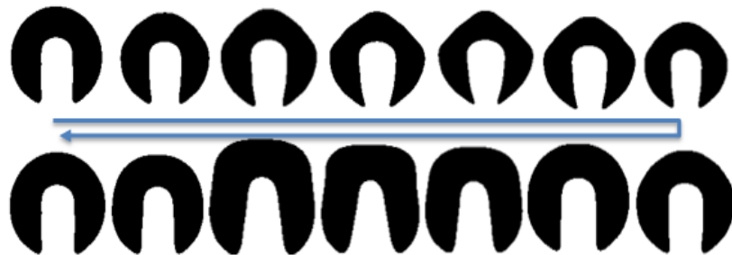
Figure 18: Typical one cycle forced shape variation associated with a single PC (PC 4 in this case)
