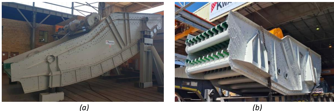
(a) (b) Figure 3: Multi-slope banana screens a) single, b) double deck [3]
