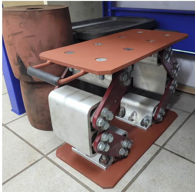
Figure 89: Resatec CH8-160 in parallel for quasi-static testing
