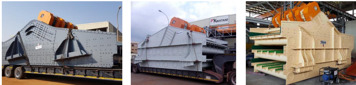
(a) (b) (c) Figure 2: Horizontal screens a) single, b) double and c) triple deck [3]
