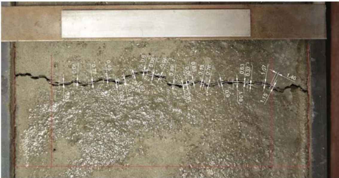
Fig. 2. Crack area calculation for a uniform crack
