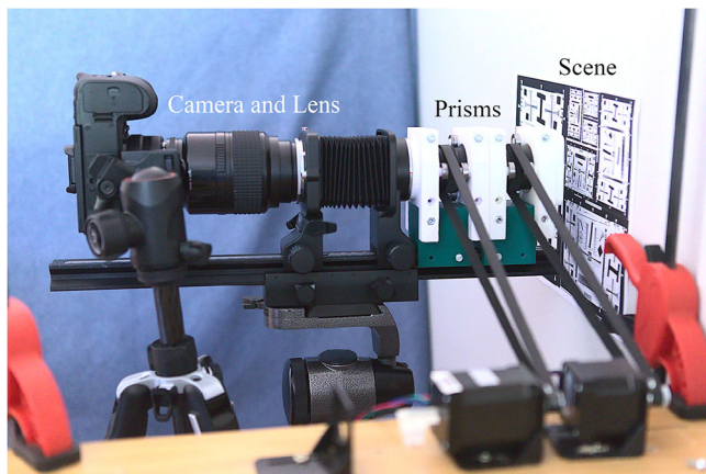
Fig. 3 A photograph of the proof-of-concept prototype of the rosette-scan TOSCA single-pixel imager
