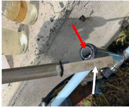
Figure S1 Stainless steel mesh (white arrow) removed from the coupon rack (indicated with a red arrow).
