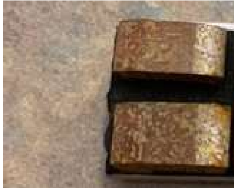
Figure S8 An example of the carbon steel coupons removed from the bacterial media on day 3, revealing the spatial arrangement of the biofilm on the surface.
