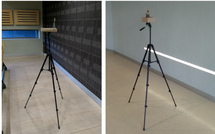
Figure 4.6. Example of TTW scenario. Anchor and tag on opposite sides of a wall.
