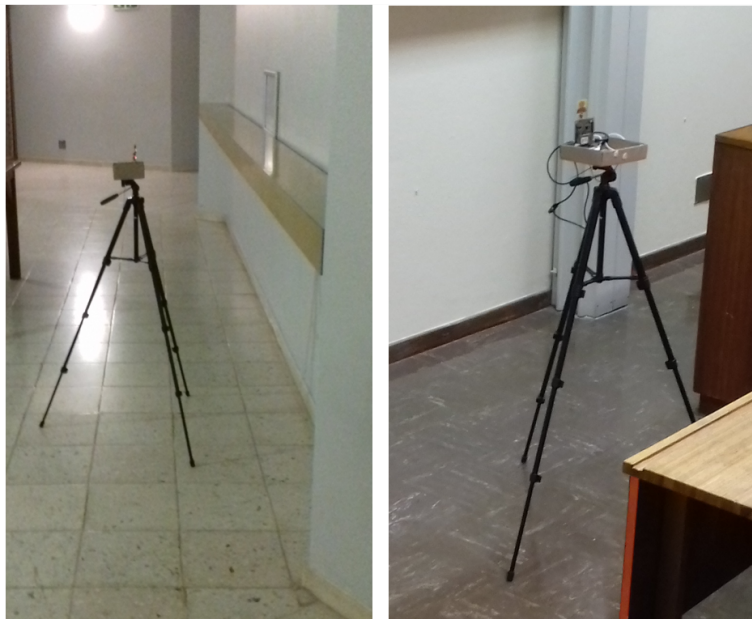
Figure 5.7. TTW ranging experiment: a tag placed in a corridor (left) and an anchor placed in a lecture hall (right). Taken from [80], © 2020 IEEE.
