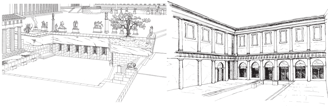
Figure 3.18. Left: Peirene Fountain, Corinth, Greece, Hellenistic period (Robinson 2013:348, following G.P. Stevens). A series of parallel walls defined six antechambers from which water was drawn, supporting the in situ rock above. The site was believed to be the place where Bellerephon tamed Pegasus, and sacred to the Muses.
