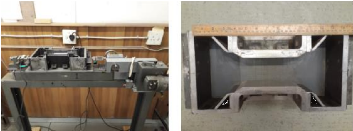
Figure 3-10: (a) Direct tensile strength apparatus and (b) Mould for direct tensile specimens
