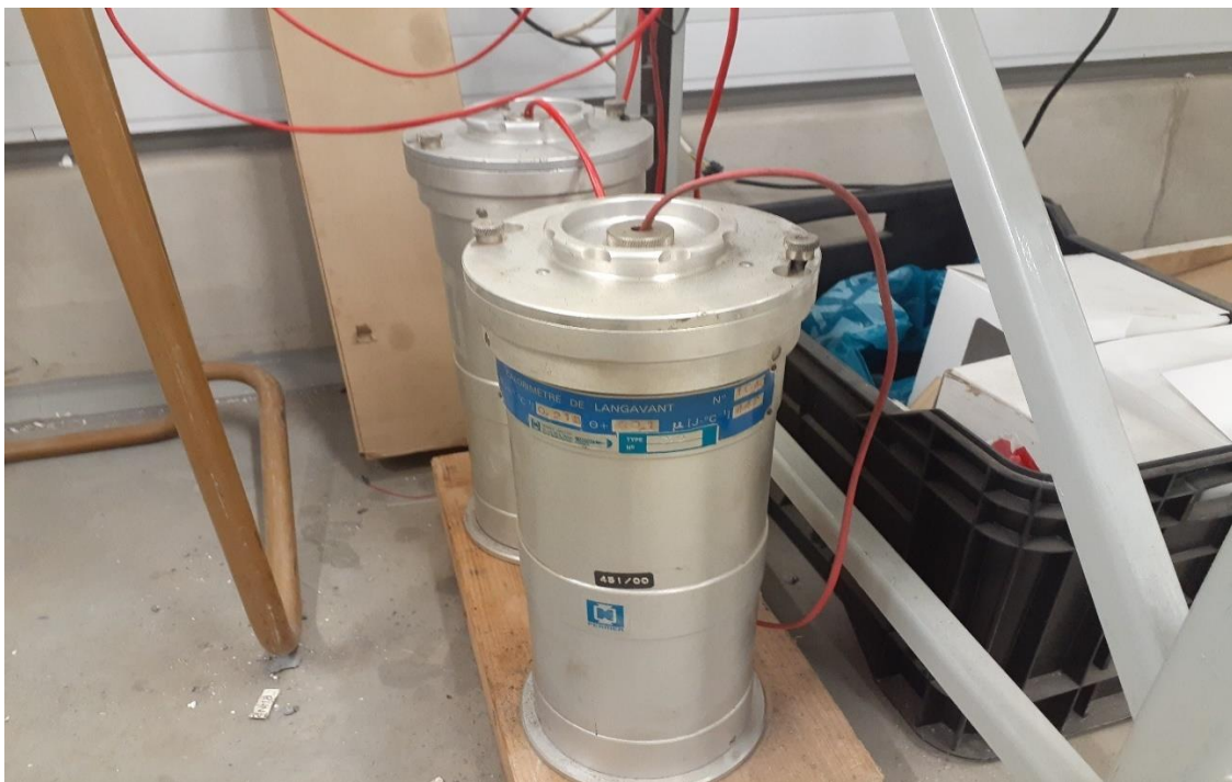
Figure 3-5: The Langevant test flask for testing the semi adiabatic heat of hydration
