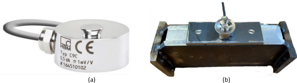
Figure 5.6: (a) A photograph of the 10 kN C9C Force Transducer, (b) a photograph of the force transducer mounted into a holder.
