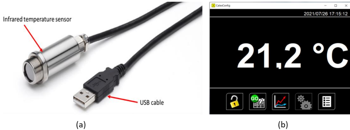
Figure 5.8: (a) PyroMiniUSB Infrared temperature sensor and (b) CalexConfig data acquisition software display.
