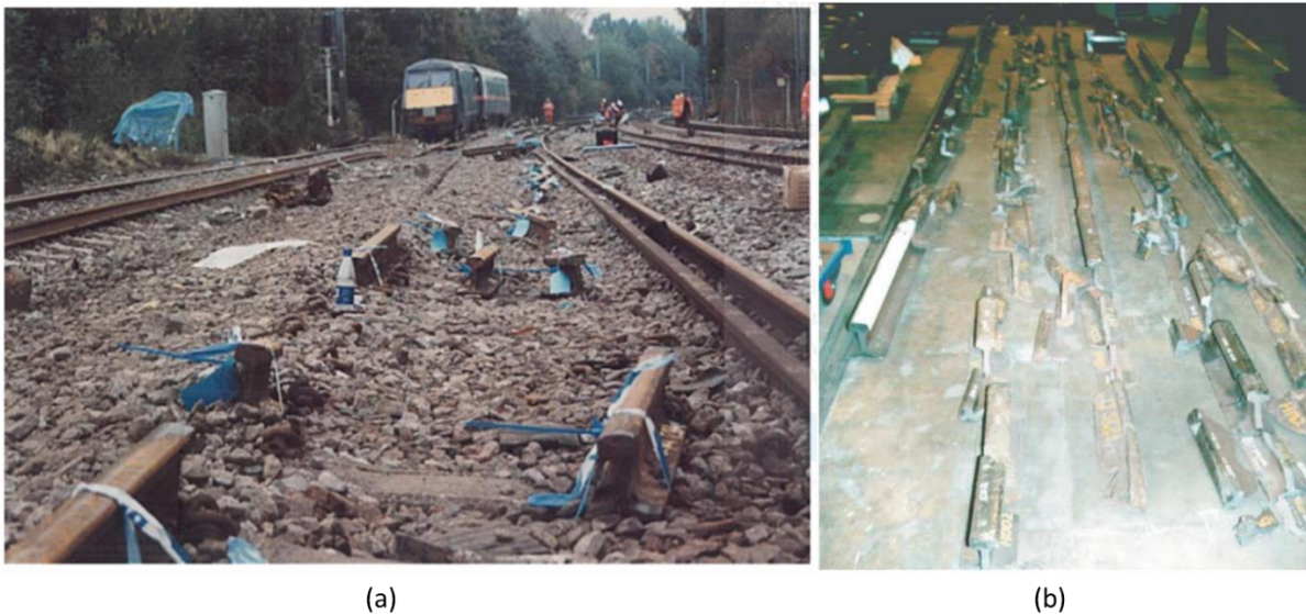
Figure 4.12: (a) The crash site at Hatfield (UK), showing disintegrated rail [154], (b) fragmented rail due to fractures from multiple rolling contact fatigue cracks [25].
