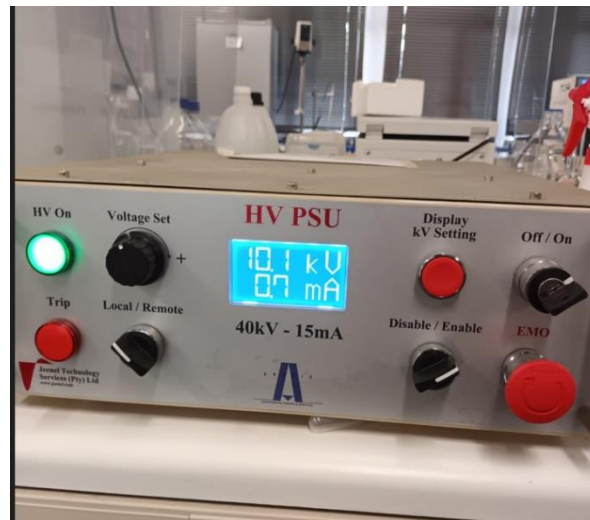
Figure B 6: Power supply for the NTP reactor
