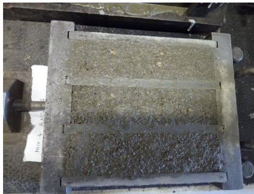
Figure 6-1: Mixed Mortar in Prism Mould
