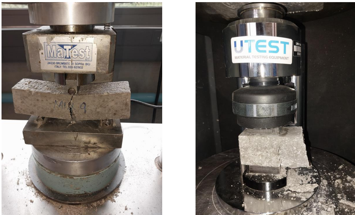
Figure A6.1: Tensile (left) and compressive (right) strength test in progress.
