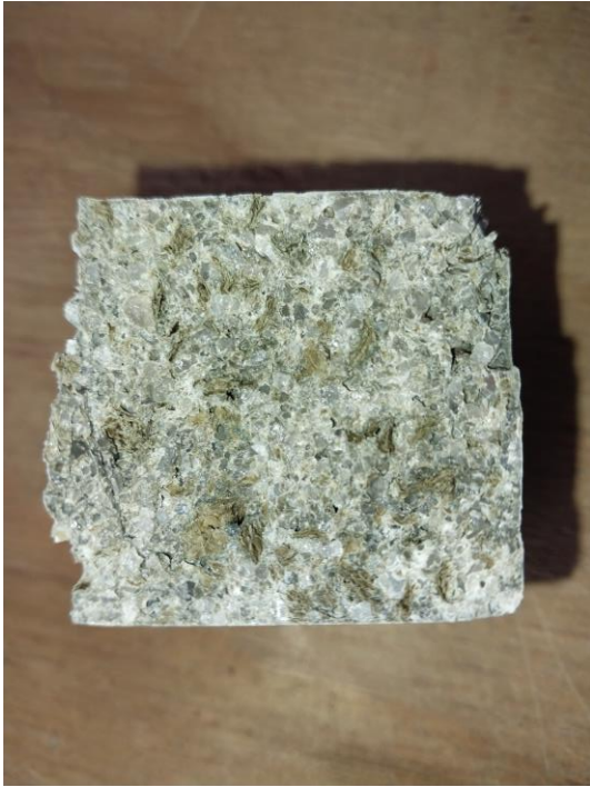
Figure A6.2: A section of the tested mortar showing imbedded membrane composite.
