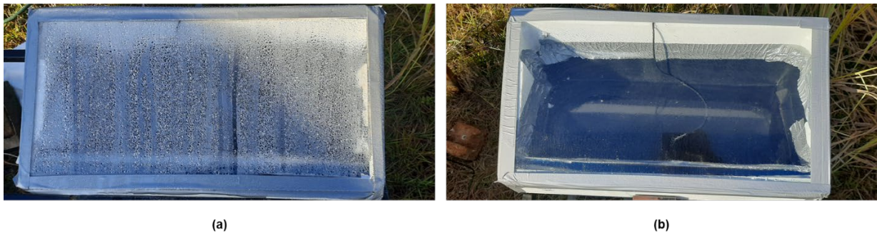
Figure 25: Comparison of condensation mechanisms for (a) PMMA and (b) Single pane glass
