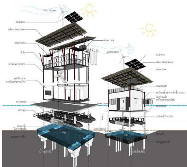
Figure 7.26. Exploded view of the amphibious house (Site Specific, 2011)
