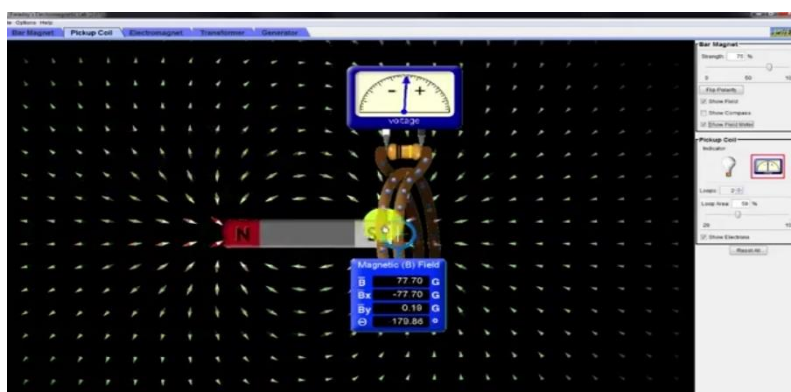
Figure 4.2.23 Screenshot from simulation showing deflection of voltmeter when a magnet moves into the coil. Source: Researcher's own.
