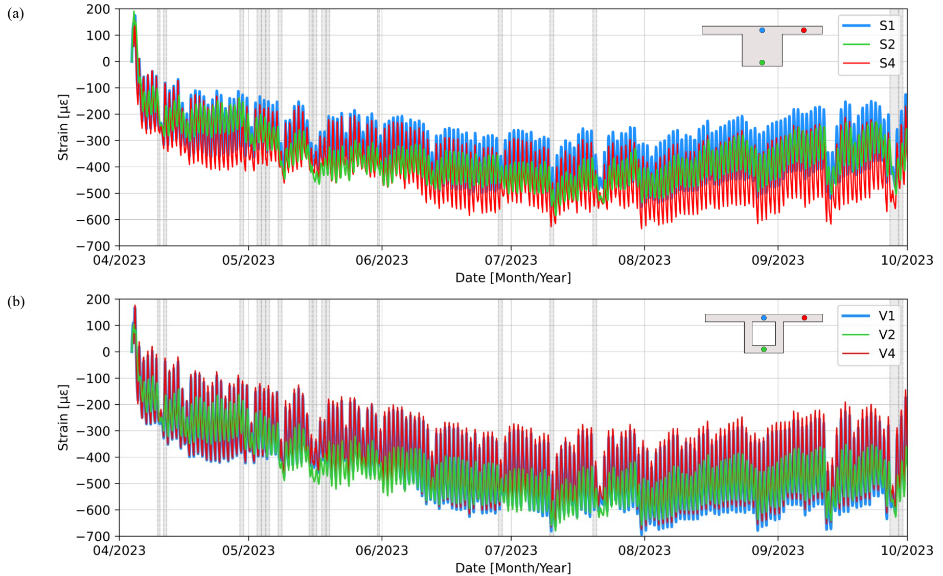
Figure 4-5 Total measured strains at selected positions of the (a) solid and (b) voided T-beam
