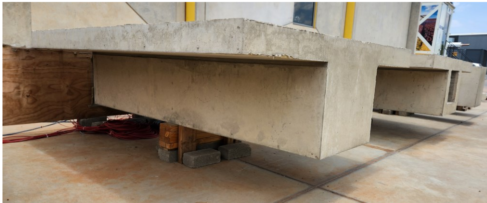
Figure 3-21 T-beams in cantilever configuration
