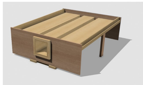
Figure 3-4 Voided T-beam mould 3D rendering
