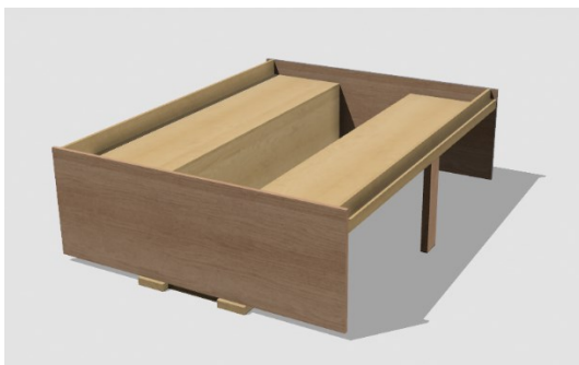
Figure 3-3 Solid T-beam mould 3D rendering
