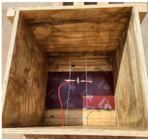
Figure 3-25 VWSG in unreinforced 0.5 m cube for CTE
