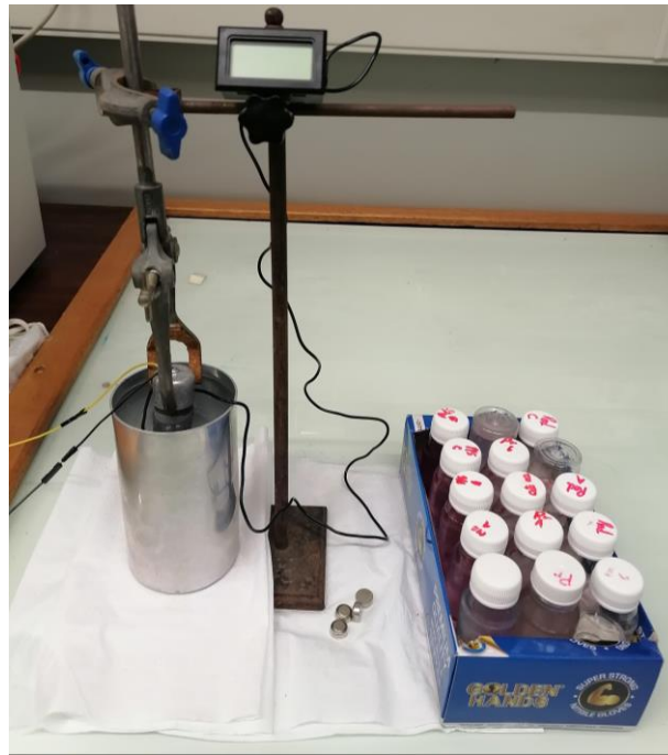
Figure 3-5: The actual experimental thermal conductivity cell device.
