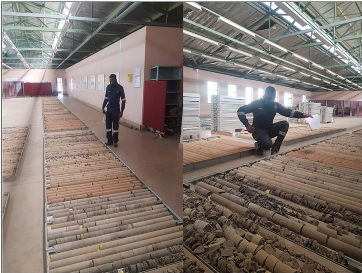
Figure 10. Core trays laid out at the national core library for logging and sampling. Generally, mudstone is broken and disaggregated while the sandstones are still intact.
