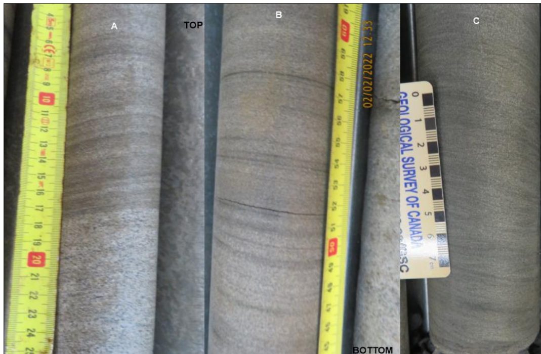
Figure 17. (A) Cross-stratification Sp stratification sandstone, core: PP5/86. (B) Horizontal Sh stratification sandstone, core: PP5/86). (C) Ripple wave Sr stratification sandstone, core: (BL1/85). Tape Measure scale is in centimeters.
