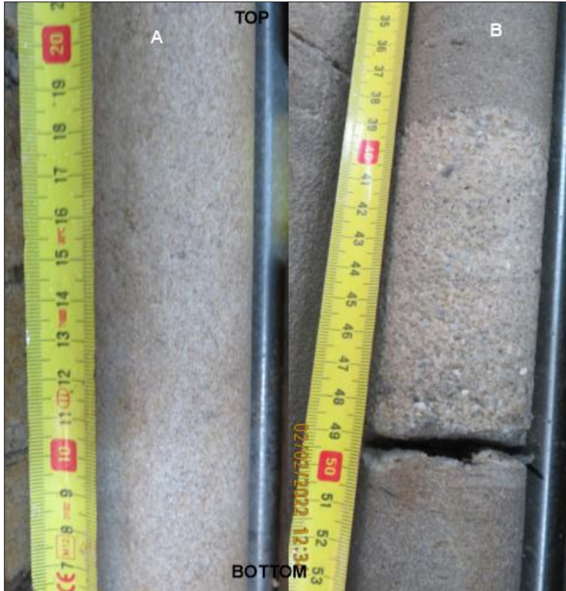
Figure 18. (A) Massive or faintly stratification sandstone, core: RF1/85. (B) Normal grading sandstone, core: MF1/85). Tape Measure scale is in centimetres.
