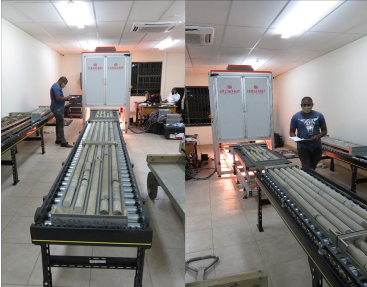
Figure 12. An image of the core trays scanned at the national core library using a hyperspectral-imaging scanner.
