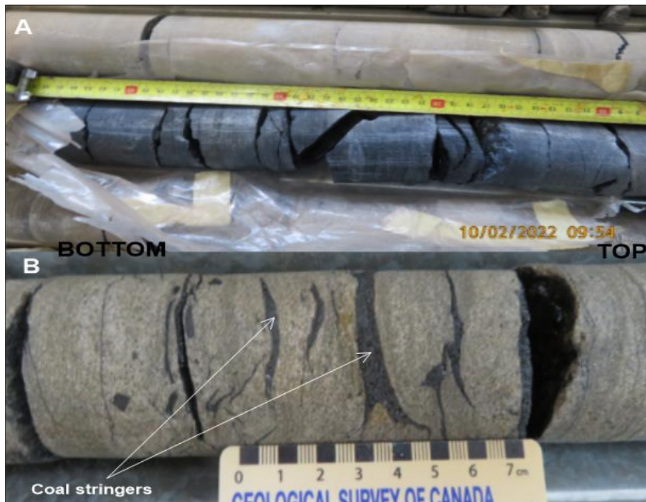
Figure 19. (A) The Guba Seam observed on core: MFI/85). (B) Vestigial coal stringers in the medium-grained sandstone (Core: BL1/85). Tape Measure scale is in centimeters.
