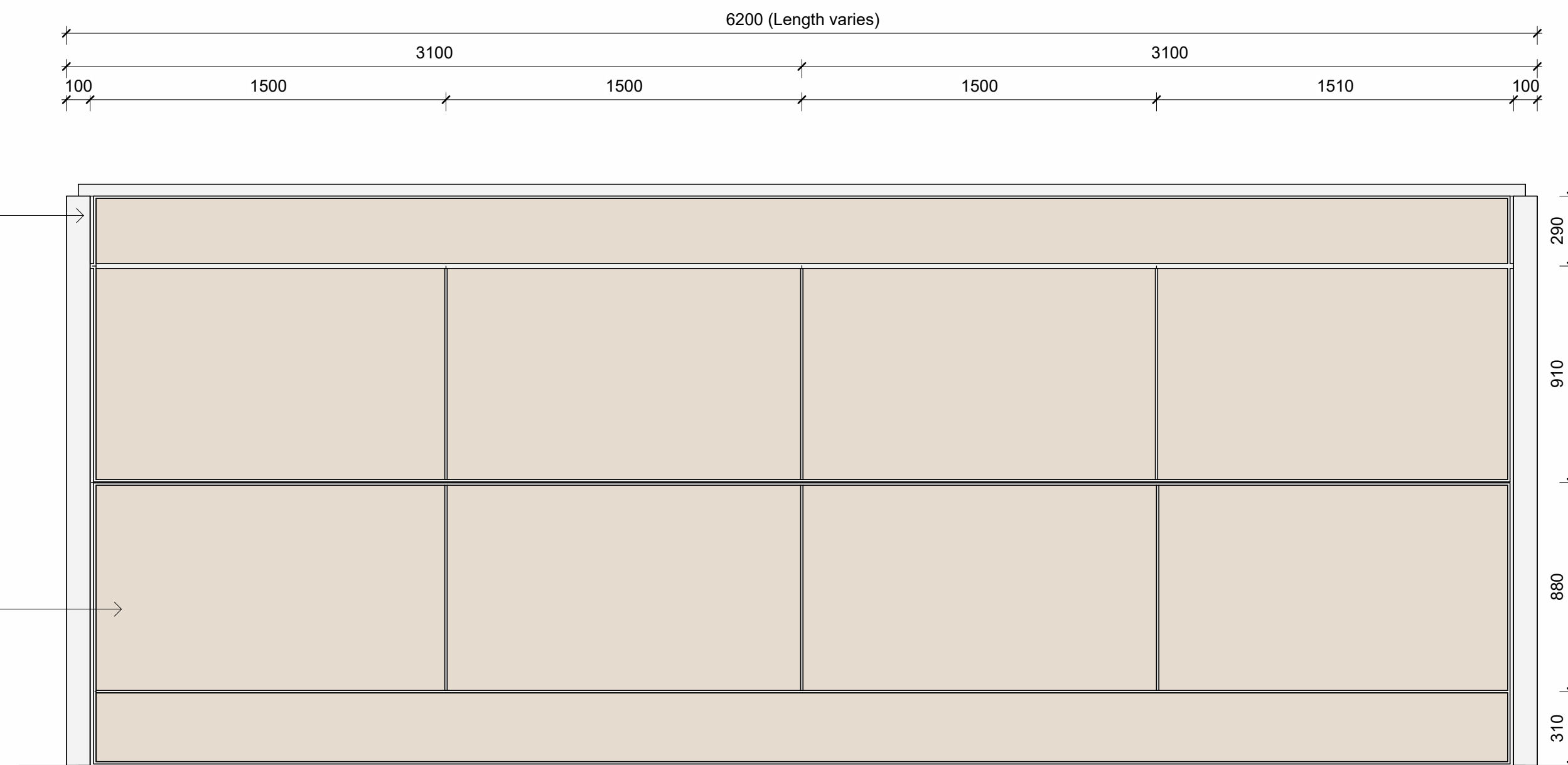
16 Elevation Front_Typical Detail_Closed 1: 20
