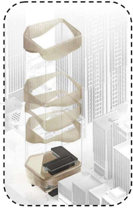
THIS BUILDING FEATURES A FAÇADE MADE UP OF 4 LAYERS THAT ALL MOVE IN OPPOSITE DIRECTIONS
