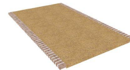
soil cement compacted in between brick paver header course
