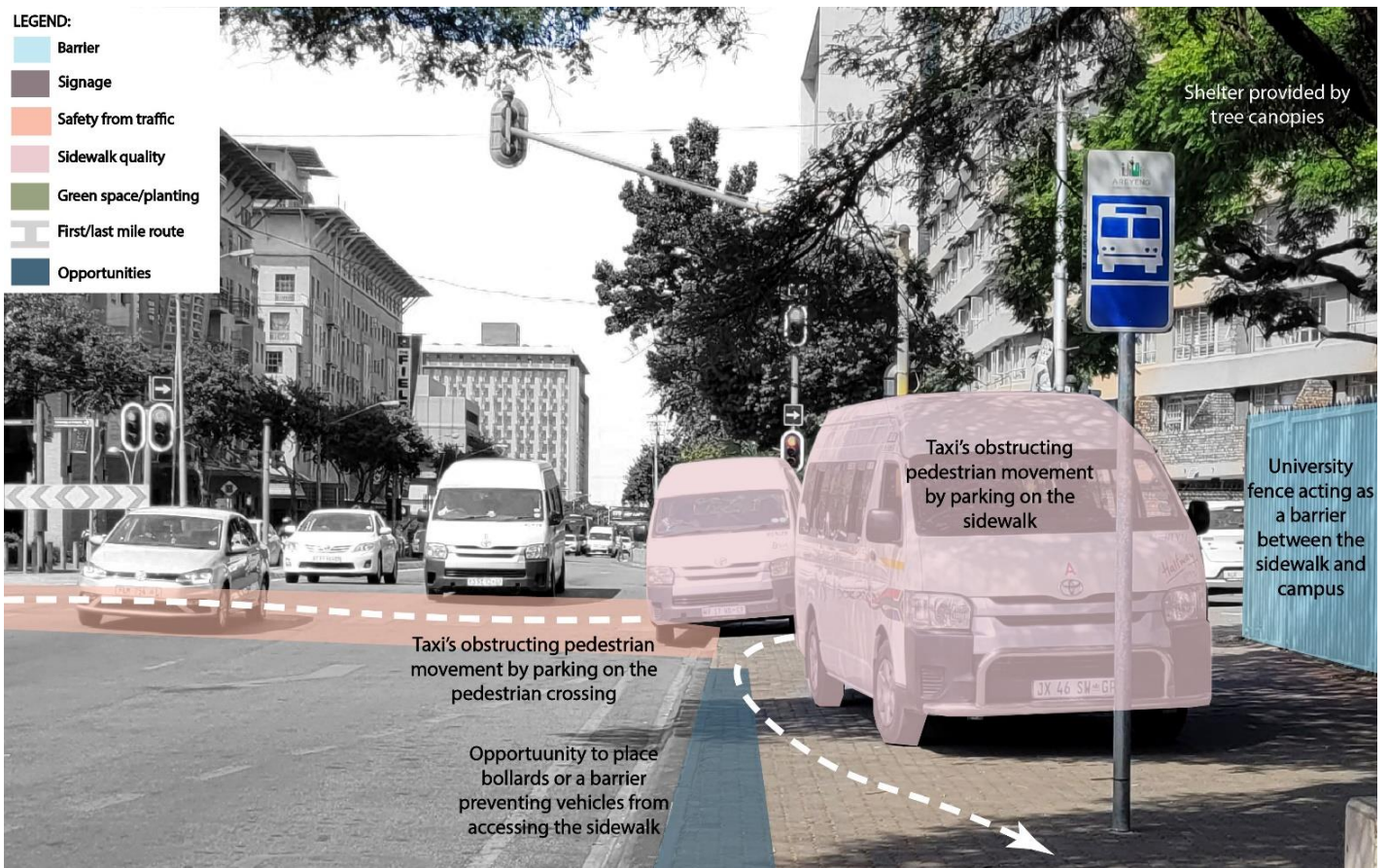
Figure 19 (Perspective E): Photographic data along Burnett Street demonstrating how taxi's park on the sidewalk to wait for passengers in the afternoon and therefore obstructing pedestrian movement (Author, 2023). A shared use of the stop/go BRT bus lane 20 meters down the road could improve this visible need.
