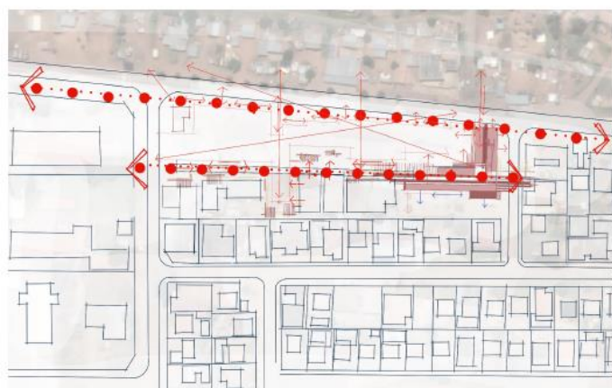
DESIRE LINES OF PED. MOVEMENT FORMING CORRIDOORS
