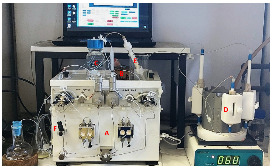
Fig S6. Reactor setup for flow bromination step with polymer bound pyridinium tribromide reagent
