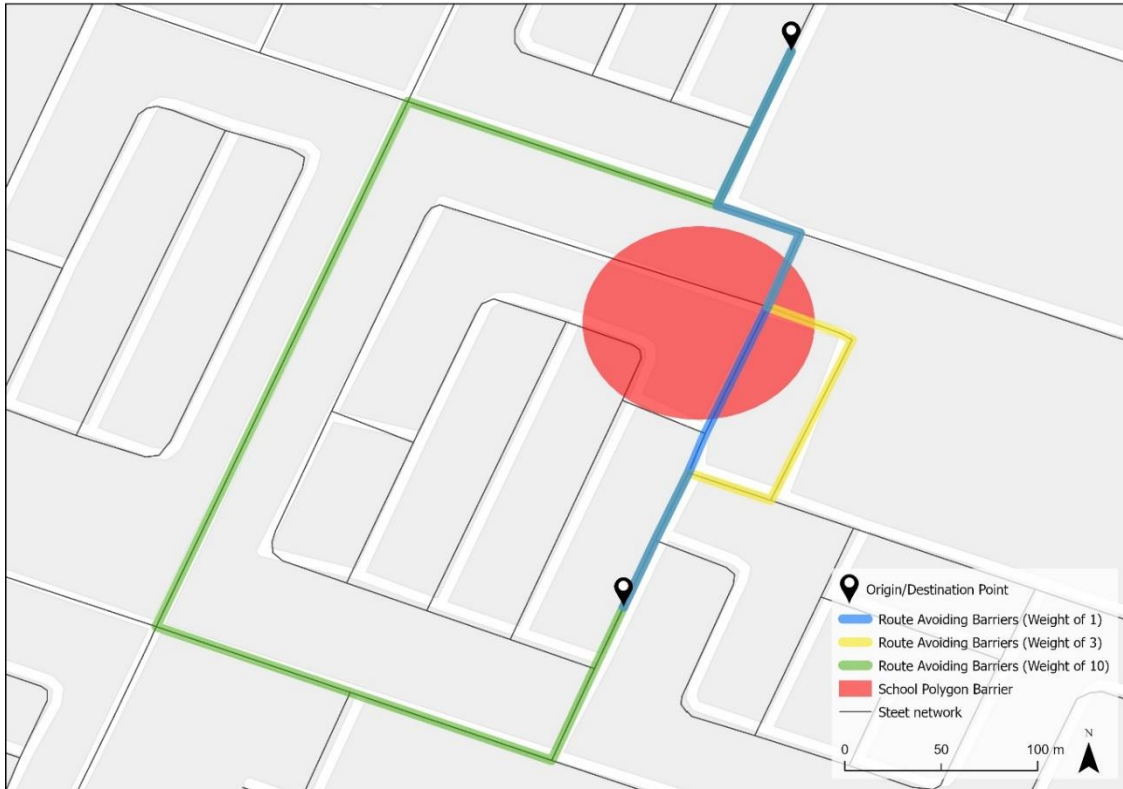
Figure 10: Map demonstrating how the weight of a school polygon barrier impacts the resultant route between two random points
